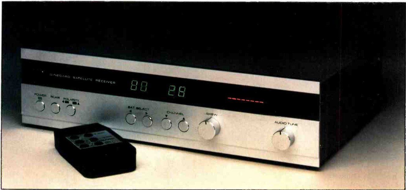
Figure 3. This TVRO receiver incorporates an infrared hand-held transmitter that enables the operator to control power on/off , polarity, satellite selection and channel selection — all from the easy chair.
