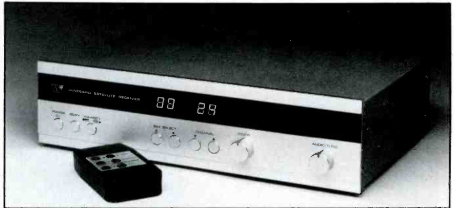
Figure 1. Front panel view of TVRO receiver with an infrared hand-held transmitter effective up to 20 feet.
