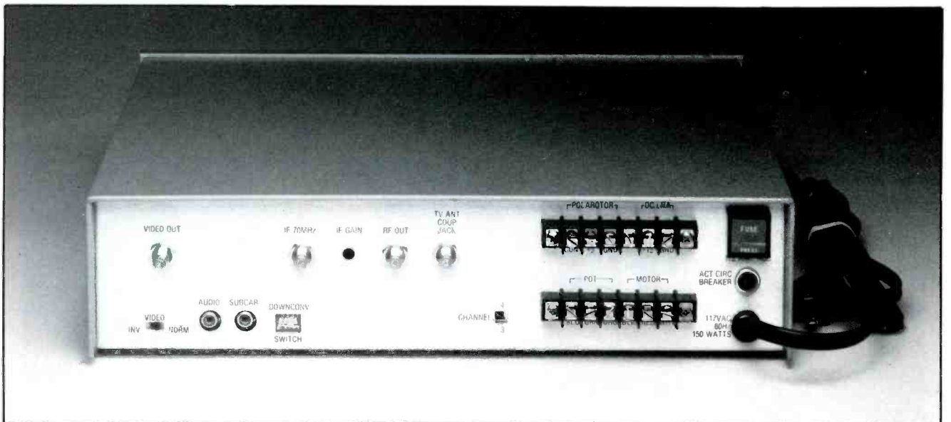
Figure 2. Rear-panel view of TVRO receiver showing input/output jacks, switches and remote-power connections.
